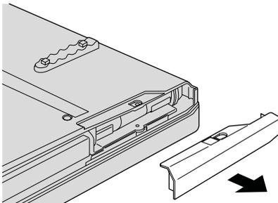
6. Remove the SSD by pulling out the tab.
