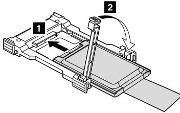
10. Insert the SSD into the slot; then press it firmly into place.
