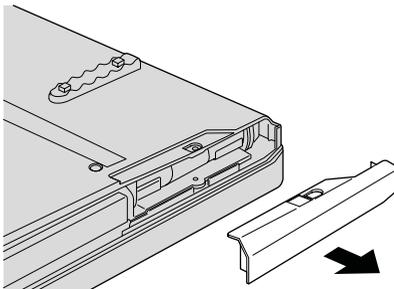
6. Remove the HDD by pulling out the tab.
