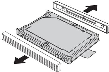
8. Attach the side rubber rails to a new HDD.
