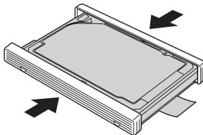
9. Insert the HDD into the slot; then press it firmly into place.
