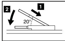
9. Pivot the SO-DIMM downward until it snaps into place.
