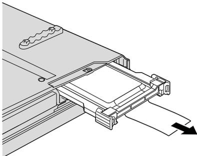
7. Release the latch with your finger in the direction shown by the arrow **1**, and lift up the bar **2**.
