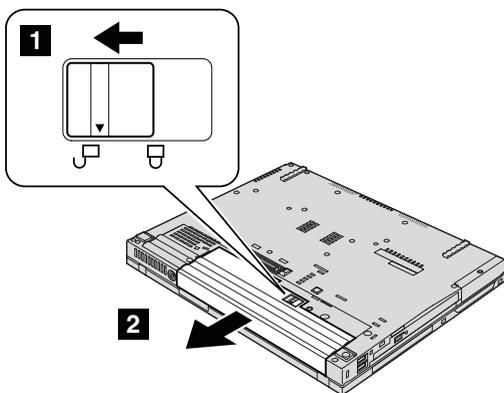
4. Install a fully charged battery.
