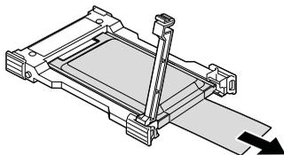
9. Insert a new SSD into the adapter **1**. Put the bar back in place and set the latch **2**.
